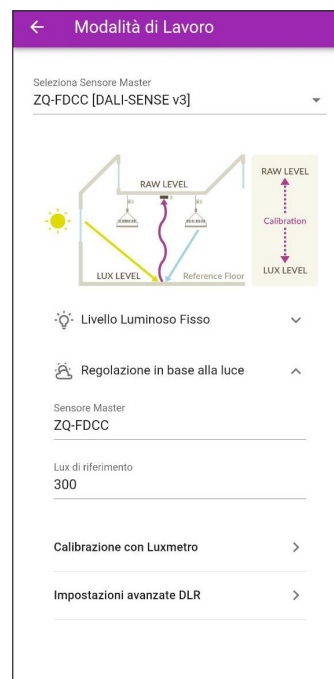
Regulation according to daylight
