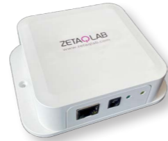
Wireless to ethernet gateway
