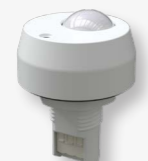
Z-PLUG-SENSOR-HB Wireless multisensor with DALI interface. Motion and light sensors for up to 17m. Powered from 12-15Vdc or via DALI bus (D4i drivers)
