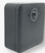
Z-SENSOR-xB R1 Wireless multisensor with DALI and 1/10 interface for max 32 drivers. 5A power relay. Motion and light sensors for up to 17m. Powered from 110-240Vac or via DALI bus (D4i drivers)
